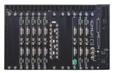
The preconfigured FSN3G-1004 is a fully integrated multi-screen presentation system that simplifies system interconnections, setup and control while providing advanced features for presentations with up to four independent screens.
