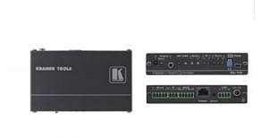
The SL-1N is a master room controller that can operate over Ethernet (LAN) with control ports that include two bidirectional RS-232, two IR and three relay. It controls devices such as scalers, video displays, audio amplifiers, DVD players, sensors, screens, shades, door locks, and lights. Multiple Kramer Ethernet gateways can be used to add remote I/O ports.
