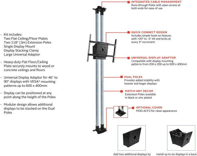
Add two additional displays by adding two Single Display Mount accessories, MOD-FPMS2, and Stacking Clamps, MOD-ASC2 (MOD-UNL2 may be required).
