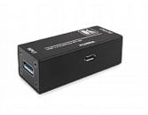
PT-3U is an innovative active USB 3.0 extender that extends the USB cable distance between the host and the device by reclocking and equalizing the USB signal. Placing PT-3U in the transmission path, removes dropout and digital noise (sparkles) in your installation that may result from using long USB cables
