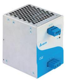
The PRA-PSM48 power supply module is a compact DIN-rail mounted power supply, delivering 48 V at up to 5 A continuously. This power supply is an OEM power supply, made for Bosch by Delta Power Supply, as a cost effective alternative to the PRAESENSA multifunction power supply PRA-MPS3 to power a PRAESENSA power amplifier in case the additional functions and characteristics of the multifunction power supply are not needed. It is not certified for EN 54-4 and similar standards.
