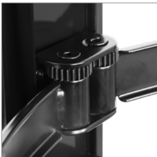
Integrating, toothed wheels allow the arms to adjust in unison, symmetrically to the centre of the mount
