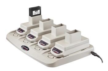
The CHG-1800 LI4 is a 4-bay full-featured battery charger for the RTS BP-240 Lithium Ion battery. This battery pack is utilized by the TR-1800 and TR-240 beltpacks. The charger offers status indicators and rapid charge capability. The CHG-1800 LI4 also offers "Intelligent Charging" optimizing the battery charge cycle and maintains the battery pack at peak capacity indefinitely.
