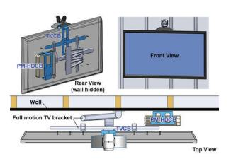
The HD codec bracket model **PM-HDCB** allows you to easily install your video conferencing codec in multiple configurations and locations. Whether you want the codec hidden behind the TV or right out front, left, right or upside down. Its design securely attaches codecs to any of our PM-Series mounts or any wooden/MDF cart while allowing airflow space between the two. Constructed from durable 11ga steel and powder coated black, it completes the HD video conferencing install.
