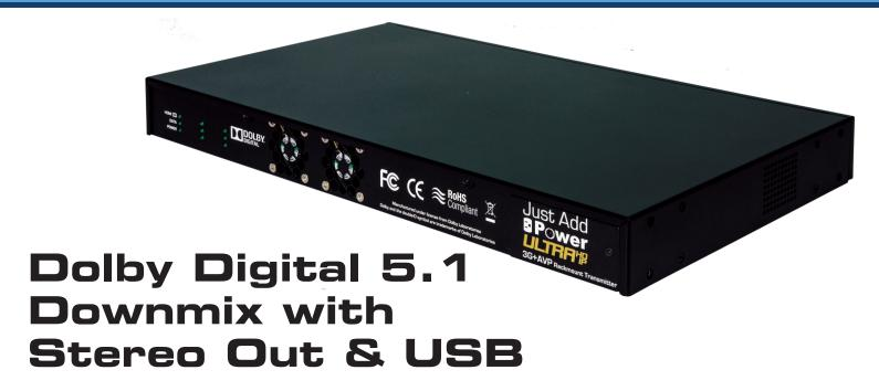
The 3G Ultra 749A Rackmount 3-in-1 Transmitter distributes 4K video over a single Cat5e cable, along with Dolby Digital 5.1.
