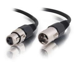
Use this XLR to XLR cable to connect unbalanced sources to balanced XLR inputs. This pro-audio cable is made from 22 AWG twisted pair audio cable under an aluminum foil shield and 60% copper braid for maximum shielding from noise. The highly flexible 7mm PVC jacket reduces the risk of the cable kinking and damaging the conductors.
