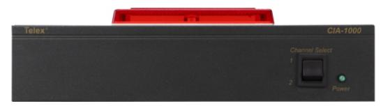
The CIA-1000 Call Indicator Assembly connects to a RTS TW intercom channels and provides an attention-getting indicator light for cueing and paging. The light can be activated by any call button on the channel. Relay contacts are also included for activation of an external device along with the light.
