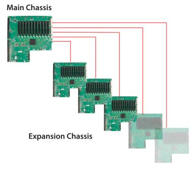
All PCI Express slots in the master chassis (containing the SBC) can be populated with a HLink-G3 card. Each HLink-G3 is then connected to an expansion chassis using an ExCable-G3 and SLink-G3 card. This configuration provides a high number of available PCI Express slots supporting low latency. The Express11-G3 can also be used to connect a mixture of multiple Datapath Express9-G3 and Express11-G3 backplanes.
