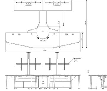
The VC-TABLE T4 Package consists of 1x VC-TABLE + 2x CR3000EX credenza + 2x PM2-S or 2X PM2-XL monitor mount. VC-TABLE T4 provides up to 82 rack units. Designed primarily for the telepresence market, this table features cable management and grommets/cubby's for easy plug in of laptops or USB keys and displaying on screen. The VC-TABLE built-in equipment rack can house a codec or PC with ten rack units easily accessible from front and rear.
