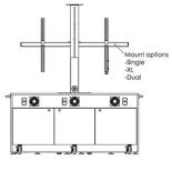
The VC-TABLE T3 Package consists of 1x VC-TABLE + 1x CR3000EX credenza + 1x PM2-D or PM2-S-XL monitor mount. VC-TABLE T3 supports ups to 46 rack units. Designed primarily for the video conference market, this table features cable management and grommets/cubby's for easy plug in of laptops or USB keys and displaying on screen. The VC-TABLE built-in equipment rack can house a codec or PC with ten rack units easily accessible from front and rear.
