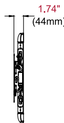
SIDE VIEW COLLAPSED
